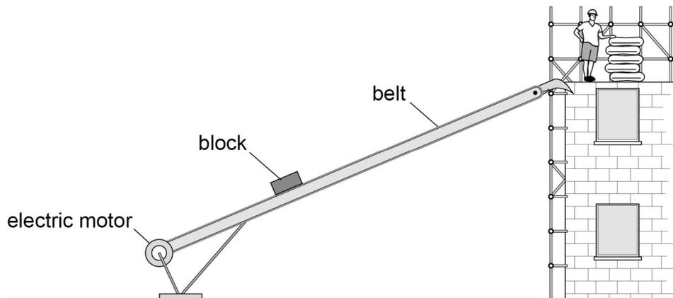
**Figure 11** shows an enlarged view of one block on the belt. The belt is inclined at  $23^\circ$  to the horizontal. The mass of the block is 19 kg.
