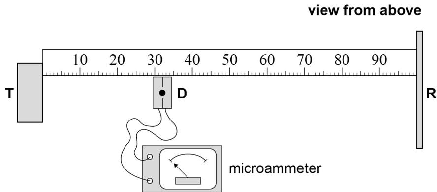
The student places a microwave detector **D** approximately one-third of the distance from **T** to **R**. When **T** is switched off, the microammeter connected to **D** reads zero.
