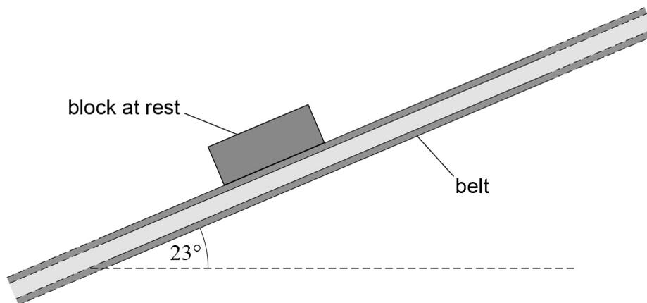
The belt exerts a frictional force  $F$  on the block when the block is at rest.
