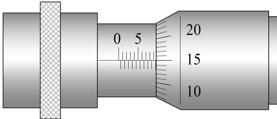
main scale and micrometer scale
